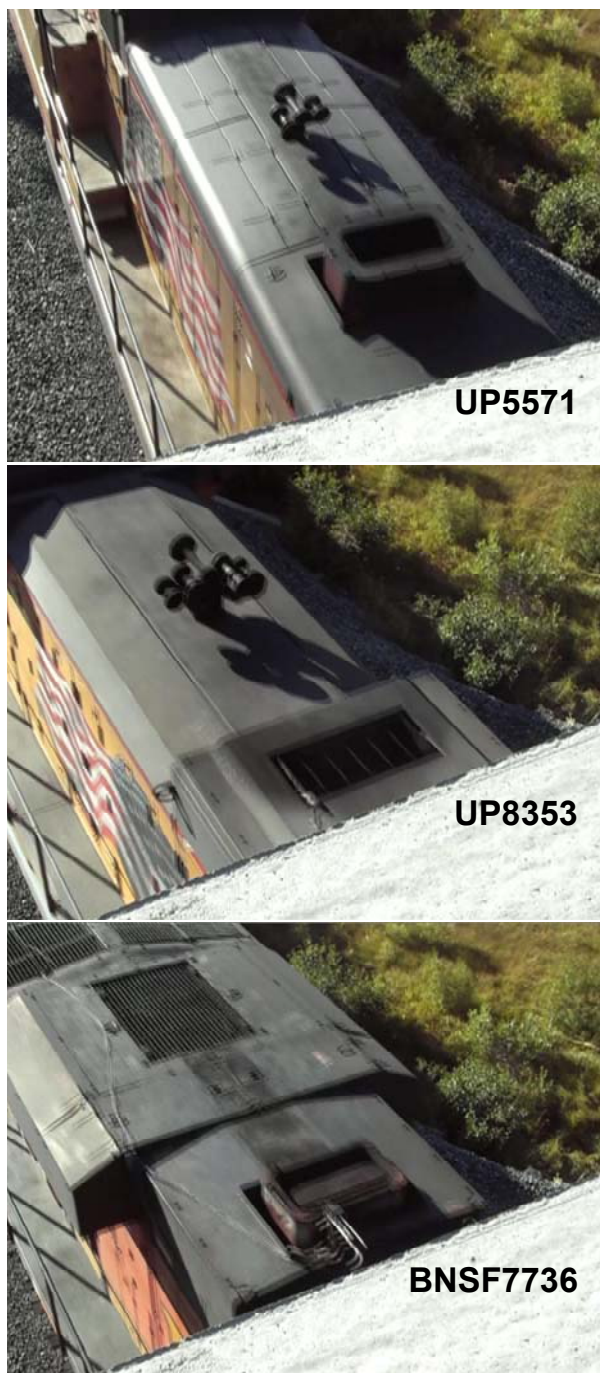
Figure 7: Exhaust stack configurations for UP5571 (UP5559 was identical), UP8353 and BNSF7736.
