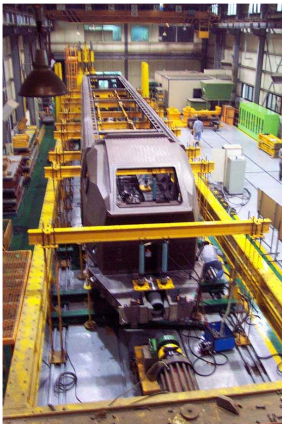
Figure 6: Load test of a power car
