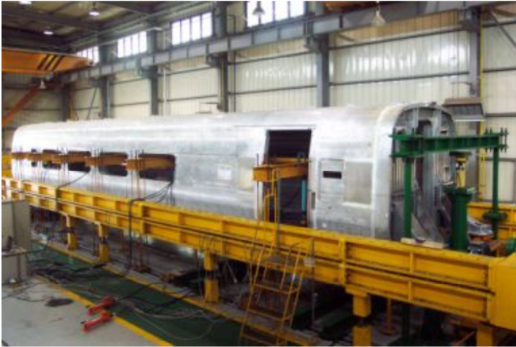
Figure 7: Load test of a trailer car
